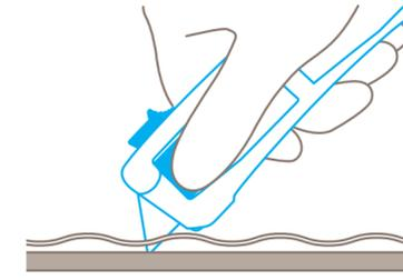
When cutting film, be sure there is **enough counter-pressure** that the blade does not retract by itself.
