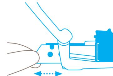
Now either **rotate or change the blade**, before pulling the blade carrier back into its original position.
