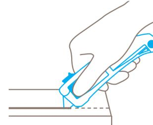
It is safe to leave your **thumb on the slider** whilst cutting.
