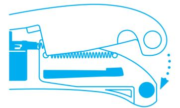
Finally, fold the **upper half of the handle back down** until it snaps into place. Please check blade retraction!
