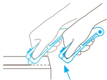
The blade automatically retracts into the handle the moment cutting ceases. Even when the slider is still **being held forwards**.
