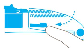
Release the blade carrier by **pressing down and pushing forward**, as indicated.
