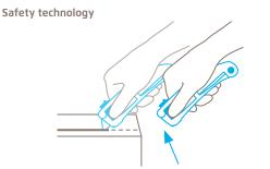
**Fully automatic blade retraction – a very high degree of safety** The fully automatic blade retraction of the SECUPRO MAXISAFE guarantees a very high degree of safety from cut injuries. The blade withdraws into the handle the moment it leaves the material being cut. Even when the slider is being held forward.
