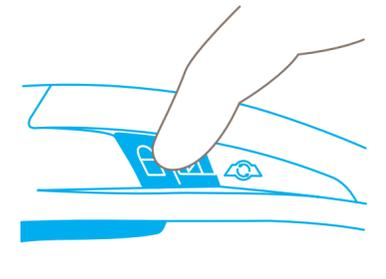
To prevent unintentional blade activation, always **lock the safety knife** by pressing downwards on the lock symbol.
