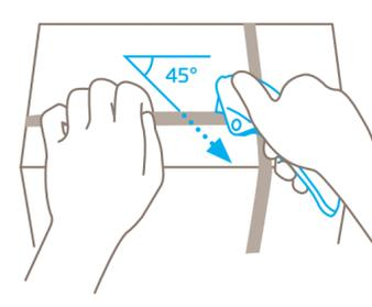
For best results, cut plastic strapping band **diagonally** (at a 45° angle).
