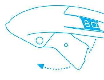
**Swing the lever out** of the handle and flip open the blade cover.
