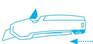
Secure the lever with the safety device and turn the handle so that the **transparent blade cover is facing upwards**.
