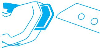
Now **reverse or change** the blade. Make sure that the blade is exactly positioned on the cams on the blade holder.
