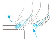
Automatic blade retraction – a high degree of safety
