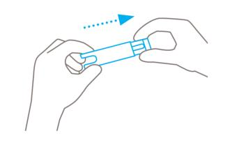
Pull plastic part out of handle's end. **Don't** pull the insert while holding onto the slider.
