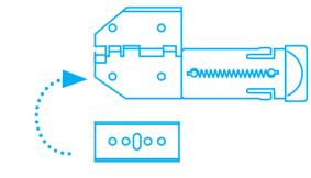
Reverse or replace the blade, make sure it fits **exactly** over the locating lugs.
