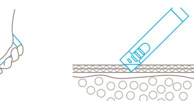
Following cutting, the blade immediately retracts into the handle. Condition: you have released hold of the slider.
