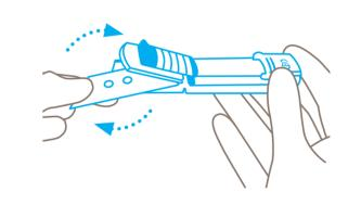
Reverse or replace the blade. Make sure you place the blade **exactly on the locating lobes**. Left-handers turn the blade 180°.
