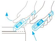
Automatic blade retraction – a high degree of safety The automatic blade retraction of the SECUNORM 525 guarantees a high degree of safety from cut injuries. As soon as you have started to cut, take your thumb off the slider. Then the blade will retract into the handle immediately after leaving the material being cut.
