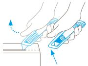
Automatic blade retraction – a high degree of safety The automatic blade retraction of the SECUNORM 500 guarantees a high degree of safety from cut injuries. As soon as you have started to cut, take your thumb off the slider. Then the blade will retract into the handle immediately after leaving the material being cut.
