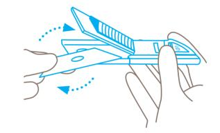
Reverse or replace the blade. Make sure you place the blade **exactly** on the locating lobe.
