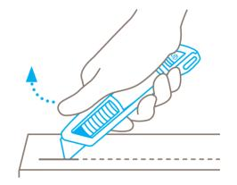
Always remove your **thumb from the slider** to ensure automatic blade retraction.
