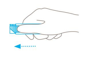
Use the slider to **engage the blade** for cut-**Pierce** into the cutting material to cut. ting.
