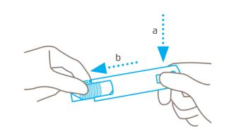
Press the blade change button downwards and at the same time pull out the slider all the way from the front.
