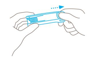
Press the blade-change button and **pull out** the plastic insert.
