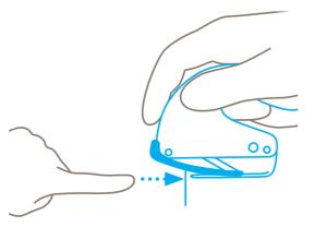
The concealed blade provides a maximum degree of **protection from cut injuries**.
