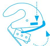
Press the catch again and insert the metal foot back into the handle until it **clicks**. Check that the foot is correctly inserted.
