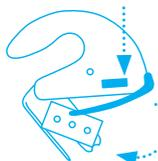
Press the catch and remove the metal foot from the handle. Replace or reverse the blade.
