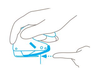
The concealed blade provides a maximum degree of **protection from cut injuries**.
