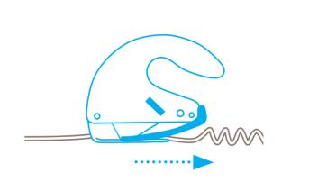
Whether cutting foam or film, the bendable plastic material-guide reliably stops material jamming in front of the blade.
