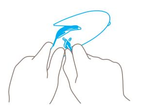
Use the locking key to lock the blade change mechanism ("lock closed").
