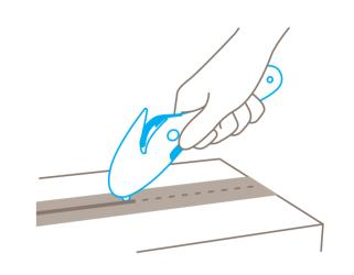
To use the **tape splitter** located at the head of the cutter, simply turn the cutter over.
