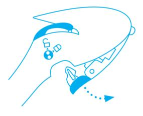
With two fingers, **disengage the blade holder** and swing it open.
