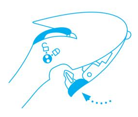
Finally, close the blade cover and push the blade holder **back into the handle**. With a click, everything is in place.
