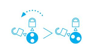
Use the locking key to **unlock the blade** change mechanism ("lock open").
