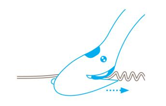
The **plastic guide** flattens the material being cut, making thin foil and paper easy to work with.
