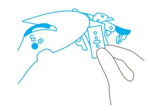
You can now lift up the blade cover to either rotate or change the blade.
