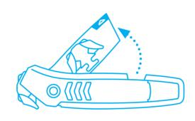
Swing open the **blade magazine**. The fitted blade head will automatically disengage.
