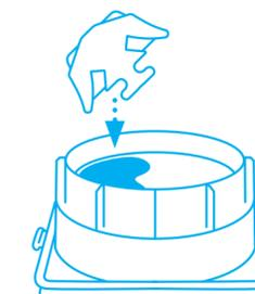
Dispose of the **used blade head** in either your **USED BLADE CONTAINER**...
