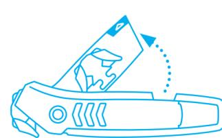
Swing open the **blade magazine**. The fitted blade head will automatically disengage.
