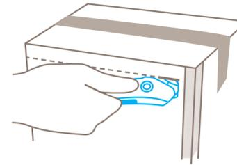
Use the nose of the cutter to **pierce** the cutting material. **Do not lever** against staples, nor force the nose into edge protectors!
