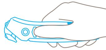
For the best possible grip, place your thumb on the **three ribs**. The soft-grip further limits the possibility of slipping.
