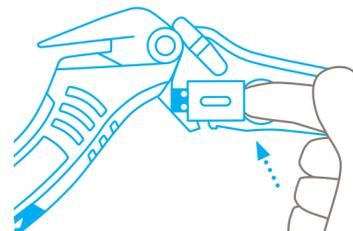
Place the thumb on the blade symbol and open up the blade cover. Remove the blade from the **side**. Turn or change the blade.
