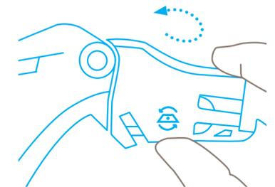
**Close** the blade cover and **fold the blade carrier back** into the handle letting the blade change button **audibly snap** into place.
