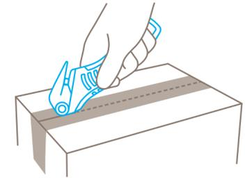
To use the **tape splitter**, turn the cutting tool around by 180 degrees.
