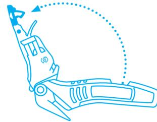
**Fully** open the blade carrier from the handle using the blade change button.
