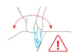
If the blade head becomes stuck, **don't force-** For best results, cut plastic strapping band fully lever the cutter!
