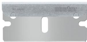
REINFORCED RAZOR BLADE NO. 60044 from MARTOR is a high-quality blade made of steel. It is very sharp and has one usable cutting edge. Rounded tips increase user safety. The blade is 39.5 mm long, 19.3 mm wide and 0.30 mm thick.
