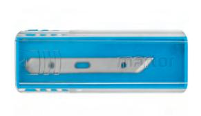
GRAPHIC BLADE NO. 606 from MARTOR is a high-quality blade made of steel. It is very sharp and has one usable cutting edge. Rounded tips increase user safety. The blade is 31.1 mm long, 5.7 mm wide and 0.50 mm thick.
