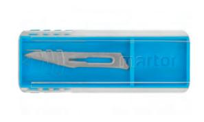
SCALPEL BLADE NO. 10 from MARTOR is a high-quality blade made of steel. It is very sharp and has one usable cutting edge. The blade is 41.7 mm long, 7.2 mm wide and 0.40 mm thick.
