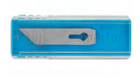
GRAPHIC BLADE NO. 677 from MARTOR is a high-quality blade made of steel. It is very sharp and has one usable cutting edge. The blade is 37 mm long, 6.1 mm wide and 0.50 mm thick.
