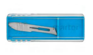
SCALPEL BLADE NO. 14 from MARTOR is a high-quality blade made of steel. It is very sharp and has one usable cutting edge. The blade is 48.8 mm long, 7.5 mm wide and 0.40 mm thick.
