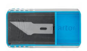
GRAPHIC BLADE NO. 629 from MARTOR is a high-quality blade made of steel. It is very sharp and has one usable cutting edge. Rounded tips increase user safety. The blade is 34.4 mm long, 5.7 mm wide and 0.50 mm thick.
