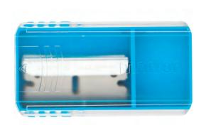
INDUSTRIAL BLADE NO. 45 from MARTOR is a high-quality blade made of steel. It is very sharp and has four cutting edges that can be used one after the other for an extra long service life. The blade is 39.0 mm long, 18.5 mm wide and 0.30 mm thick.
