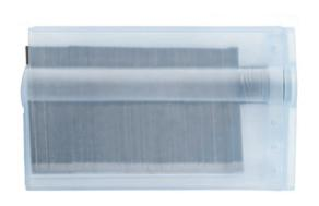
GRAPHIC BLADE NO. 8629 from MARTOR is a high-quality blade made of steel with TiN-coating. It is very sharp and has one usable cutting edge. Rounded tips increase user safety. The blade is 34.4 mm long, 5.7 mm wide and 0.50 mm thick.
