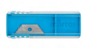
TRAPEZOID BLADE NO. 852 from MARTOR is a high-quality blade made of stainless steel with TiN-coating. It is very sharp and has two cutting edges that can be used one after the other for a long service life. The blade is 53 mm long, 19 mm wide and 0.63 mm thick. The oil used for the blade is food safe.
